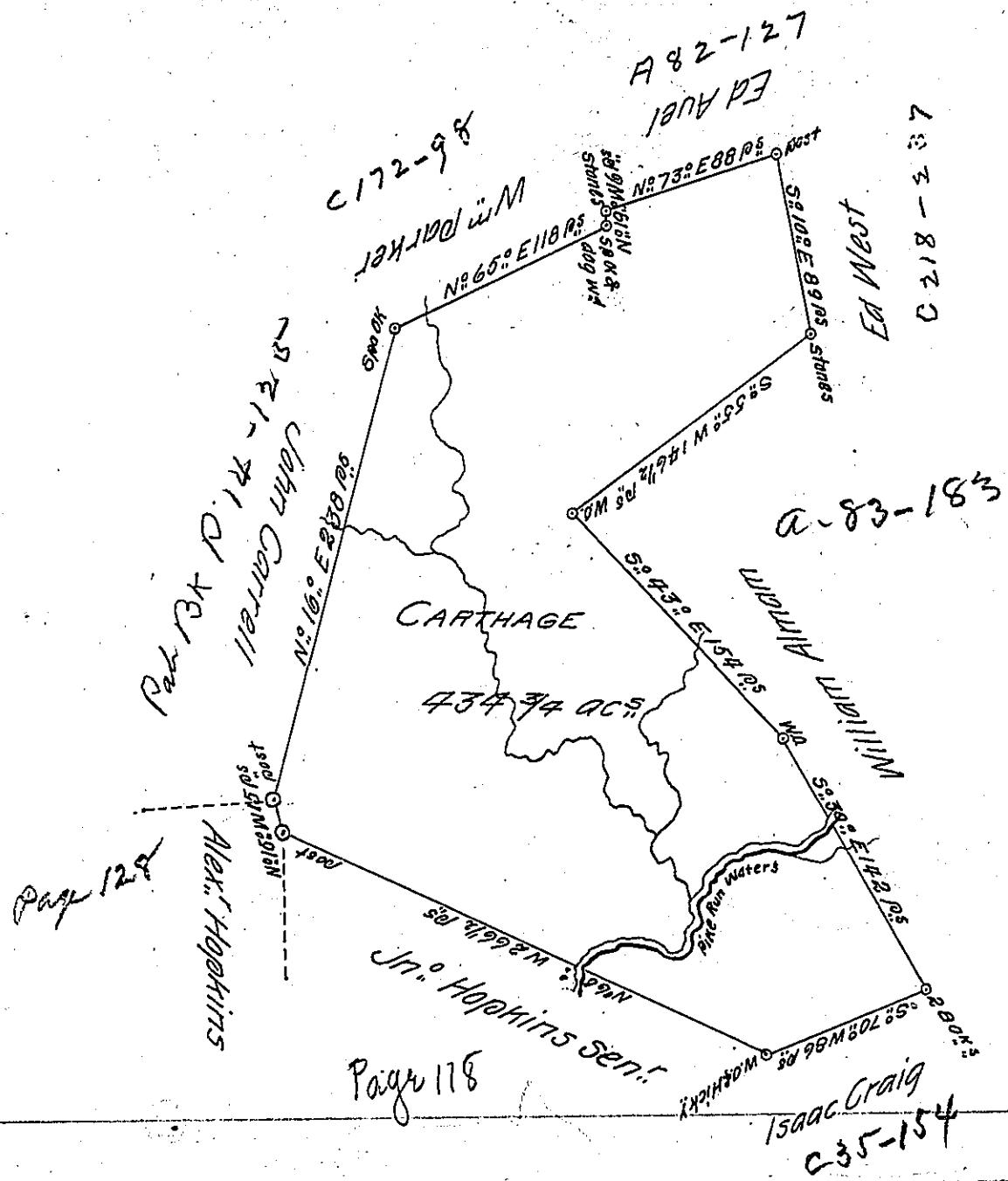
A Draught of a survey called "Carthage" situate on the waters of Pike Run in Washington County contain<sup>s</sup> 9 434  $\frac{3}{4}$  Ac.<sup>s</sup> and the usual allow<sup>ce</sup> for Roads &c. executed Apr<sup>il</sup> 23<sup>rd</sup> 1787 in pursuance of a Warr<sup>t</sup> granted to Alex<sup>d</sup> Hopkins for 700 Ac.<sup>s</sup> dated March 16<sup>th</sup> 1786
